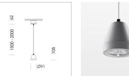
Suspended luminaire with LED, rated life of the LED L80/B10 > 50000 h, colour rendering index CRI > 95, chromaticity tolerance 2 SDCM (initial), rotation-symmetrical reflector with circular light distribution pattern, reflector pure aluminium 99,99% in MIRO-Silver®,segmented and faceted, 3D lens silicon to reduce the proportion of scattered light, luminaire head die-cast aluminium, powder-coated, stratosilver
