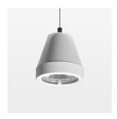
Suspended luminaire with LED, rated life of the LED L80/B10 > 50000 h, colour rendering index CRI > 80, chromaticity tolerance 3 SDCM (initial), rotation-symmetrical reflector with circular light distribution pattern, reflector pure aluminium 99,99% in MIRO-Silver®, segmented and faceted, 3D lens silicon to reduce the proportion of scattered light, luminaire head die-cast aluminium, powder-coated, stratowhite
