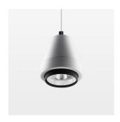
Suspended luminaire with LED, rated life of the LED L80/B10 > 50000 h, colour rendering index CRI > 80, chromaticity tolerance 2 SDCM (initial), reflector with circular light distribution pattern, reflector pure aluminium 99,99% in MIRO-Silver®, segmented and faceted, 3D lens silicon to reduce the proportion of scattered light, luminaire head die-cast aluminium, powder-coated, stratowhite
