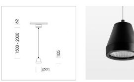
Suspended luminaire with LED, rated life of the LED L80/B10 > 50000 h, chromaticity tolerance 2 SDCM (initial), reflector with circular light distribution pattern, reflector pure aluminium 99,99% in MIRO-Silver®,segmented and faceted, 3D lens silicon to reduce the proportion of scattered light, luminaire head die-cast aluminium, powder-coated, stratoblack
