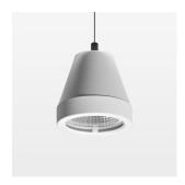
Suspended luminaire with LED, rated life of the LED L80/B10 > 50000 h, chromaticity tolerance 2 SDCM (initial), reflector with circular light distribution pattern, reflector pure aluminium 99,99% in MIRO-Silver®, segmented and faceted, 3D lens silicon to reduce the proportion of scattered light, luminaire head die-cast aluminium, powder-coated, stratowhite
