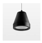
Suspended luminaire with LED, rated life of the LED L80/B10 > 50000 h, colour rendering index CRI > 80, chromaticity tolerance 2 SDCM (initial), reflector with circular light distribution pattern, reflector pure aluminium 99,99% in MIRO-Silver®, segmented and faceted, 3D lens silicon to reduce the proportion of scattered light, luminaire head die-cast aluminium, powder-coated, stratoblack
