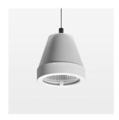
Suspended luminaire with LED, rated life of the LED L80/B10 > 50000 h, colour rendering index CRI > 90, chromaticity tolerance 2 SDCM (initial), reflector with circular light distribution pattern, reflector pure aluminium 99,99% in MIRO-Silver®, segmented and faceted, 3D lens silicon to reduce the proportion of scattered light, luminaire head die-cast aluminium, powder-coated, stratowhite
