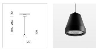
Suspended luminaire with LED, rated life of the LED L80/B10 > 50000 h, colour rendering index CRI > 96, chromaticity tolerance 3 SDCM (initial), reflector with circular light distribution pattern, reflector pure aluminium 99,99% in MIRO-Silver®,segmented and faceted, luminaire head die-cast aluminium, powder-coated, stratoblack
