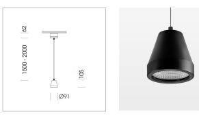
Suspended luminaire with LED, rated life of the LED L80/B10 > 50000 h, colour rendering index CRI > 90, chromaticity tolerance 2 SDCM (initial), reflector with circular light distribution pattern, reflector pure aluminium 99,99% in MIRO-Silver®,segmented and faceted, luminaire head die-cast aluminium, powder-coated, stratoblack
