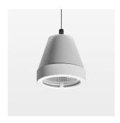
Suspended luminaire with LED, rated life of the LED L80/B10 > 50000 h, colour rendering index CRI > 90, chromaticity tolerance 2 SDCM (initial), reflector with circular light distribution pattern, reflector pure aluminium 99,99% in MIRO-Silver®, segmented and faceted, luminaire head die-cast aluminium, powder-coated, stratowhite
