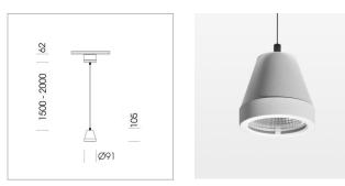
Suspended luminaire with LED, rated life of the LED L80/B10 > 50000 h, chromaticity tolerance 2 SDCM (initial), reflector with circular light distribution pattern, reflector pure aluminium 99,99% in MIRO-Silver®,segmented and faceted, luminaire head die-cast aluminium, powder-coated, stratowhite
