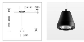
Suspended luminaire with LED, rated life of the LED L80/B10 > 50000 h, colour rendering index CRI > 90, chromaticity tolerance 3 SDCM (initial), rotation-symmetrical reflector with circular light distribution pattern, reflector pure aluminium 99,99% in MIRO-Silver®,segmented and faceted, 3D lens silicon to reduce the proportion of scattered light, luminaire head die-cast aluminium, powder-coated, stratoblack, separate driver unit
