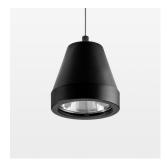
Suspended luminaire with LED, rated life of the LED L80/B10 > 50000 h, colour rendering index CRI > 95, chromaticity tolerance 2 SDCM (initial), rotation-symmetrical reflector with circular light distribution pattern, reflector pure aluminium 99,99% in MIRO-Silver®, segmented and faceted, 3D lens silicon to reduce the proportion of scattered light, luminaire head die-cast aluminium, powder-coated, stratoblack, separate driver unit
