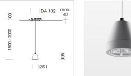
Suspended luminaire with LED, rated life of the LED L80/B10 > 50000 h, colour rendering index CRI > 80, chromaticity tolerance 3 SDCM (initial), rotation-symmetrical reflector with circular light distribution pattern, reflector pure aluminium 99,99% in MIRO-Silver®,segmented and faceted, 3D lens silicon to reduce the proportion of scattered light, luminaire head die-cast aluminium, powder-coated, stratosilver, separate driver unit
