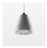
Suspended luminaire with LED, rated life of the LED L80/B10 > 50000 h, colour rendering index CRI > 95, chromaticity tolerance 2 SDCM (initial), rotation-symmetrical reflector with circular light distribution pattern, reflector pure aluminium 99,99% in MIRO-Silver®, segmented and faceted, 3D lens silicon to reduce the proportion of scattered light, luminaire head die-cast aluminium, powder-coated, stratosilver, separate driver unit
