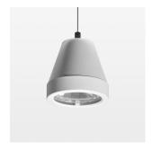
Suspended luminaire with LED, rated life of the LED L80/B10 > 50000 h, colour rendering index CRI > 90, chromaticity tolerance 3 SDCM (initial), rotation-symmetrical reflector with circular light distribution pattern, reflector pure aluminium 99,99% in MIRO-Silver®, segmented and faceted, 3D lens silicon to reduce the proportion of scattered light, luminaire head die-cast aluminium, powder-coated, stratowhite, separate driver unit
