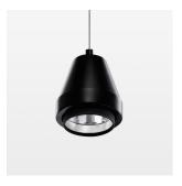
Suspended luminaire with LED, rated life of the LED L80/B10 > 50000 h, colour rendering index CRI > 80, chromaticity tolerance 2 SDCM (initial), reflector with circular light distribution pattern, reflector pure aluminium 99,99% in MIRO-Silver®, segmented and faceted, 3D lens silicon to reduce the proportion of scattered light, luminaire head die-cast aluminium, powder-coated, stratoblack, separate driver unit
