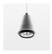
Suspended luminaire with LED, rated life of the LED L80/B10 > 50000 h, colour rendering index CRI > 90, chromaticity tolerance 2 SDCM (initial), reflector with circular light distribution pattern, reflector pure aluminium 99,99% in MIRO-Silver®, segmented and faceted, 3D lens silicon to reduce the proportion of scattered light, luminaire head die-cast aluminium, powder-coated, stratowhite, separate driver unit
