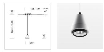
Suspended luminaire with LED, rated life of the LED L80/B10 > 50000 h, colour rendering index CRI > 96, chromaticity tolerance 3 SDCM (initial), reflector with circular light distribution pattern, reflector pure aluminium 99,99% in MIRO-Silver®,segmented and faceted, 3D lens silicon to reduce the proportion of scattered light, luminaire head die-cast aluminium, powder-coated, stratowhite, separate driver unit
