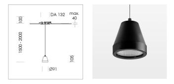
Suspended luminaire with LED, rated life of the LED L80/B10 > 50000 h, colour rendering index CRI > 90, chromaticity tolerance 2 SDCM (initial), reflector with circular light distribution pattern, reflector pure aluminium 99,99% in MIRO-Silver®,segmented and faceted, luminaire head die-cast aluminium, powder-coated, stratoblack, separate driver unit
