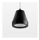
Suspended luminaire with LED, rated life of the LED L80/B10 > 50000 h, colour rendering index CRI > 96, chromaticity tolerance 3 SDCM (initial), reflector with circular light distribution pattern, reflector pure aluminium 99,99% in MIRO-Silver®, segmented and faceted, luminaire head die-cast aluminium, powder-coated, stratoblack, separate driver unit
