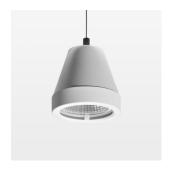
Suspended luminaire with LED, rated life of the LED L80/B10 > 50000 h, colour rendering index CRI > 80, chromaticity tolerance 2 SDCM (initial), reflector with circular light distribution pattern, reflector pure aluminium 99,99% in MIRO-Silver®, segmented and faceted, luminaire head die-cast aluminium, powder-coated, stratowhite, separate driver unit
