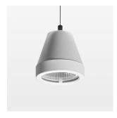
Suspended luminaire with LED, rated life of the LED L80/B10 > 50000 h, colour rendering index CRI > 96, chromaticity tolerance 3 SDCM (initial), reflector with circular light distribution pattern, reflector pure aluminium 99,99% in MIRO-Silver®, segmented and faceted, luminaire head die-cast aluminium, powder-coated, stratowhite, separate driver unit
